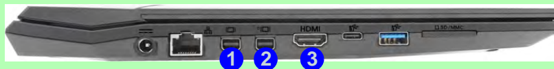
Figure C - 1 - Left Side View (Mini Display Ports & HDMI Port Highlighted) - Single Model Pictured
